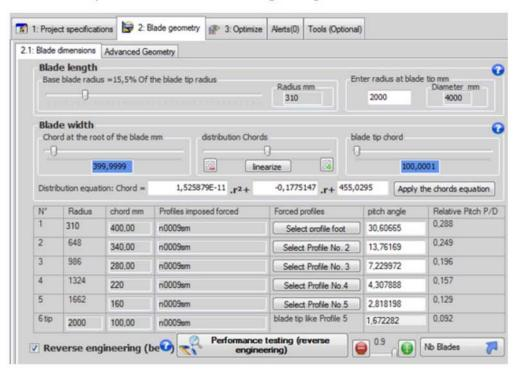
When moving in reverse engineering, some functions are not available (such as the choice of law in profile, or thickness of the profiles) because the profiles will be selected and manually forced.
