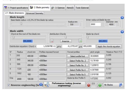
Mode, reverse engineering, is designed for testing the performance but also the reproduction of an existing propeller. You can then modify certain parameters to create a new propeller, derived from model. When you enter data pitch and geometry found on the propeller, the 3D model of the propeller may be created, you can also edit 3D files igs or solidworks for designing your prototype propeller .....
