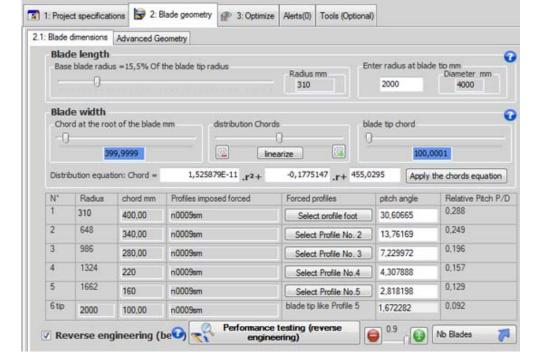
When your blade definition is complete click"performance testing (reverse engineering)". Heliciel reconstructs the <u>3d model</u> to pitch defined, then re calculating the performance of your <u>propeller</u>. You can change the <u>rotational speed</u> and <u>velocity of</u> the fluid, then repeat the test to find new performance to other operating points.
